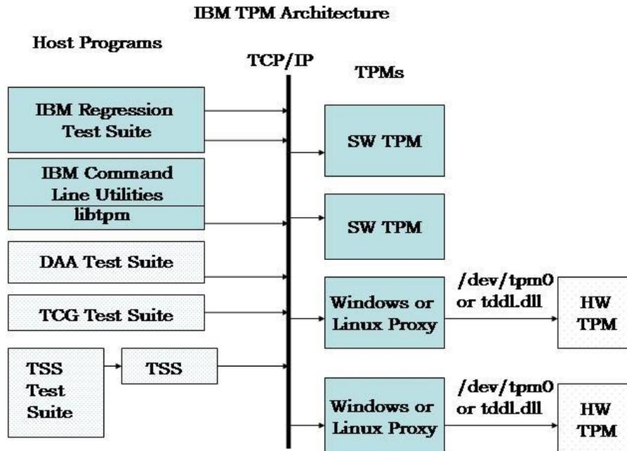
Figure 10: Architecture of IBM's TPM2.0 SW implementation (from <http://ibmswtpm.sourceforge.net/>).
