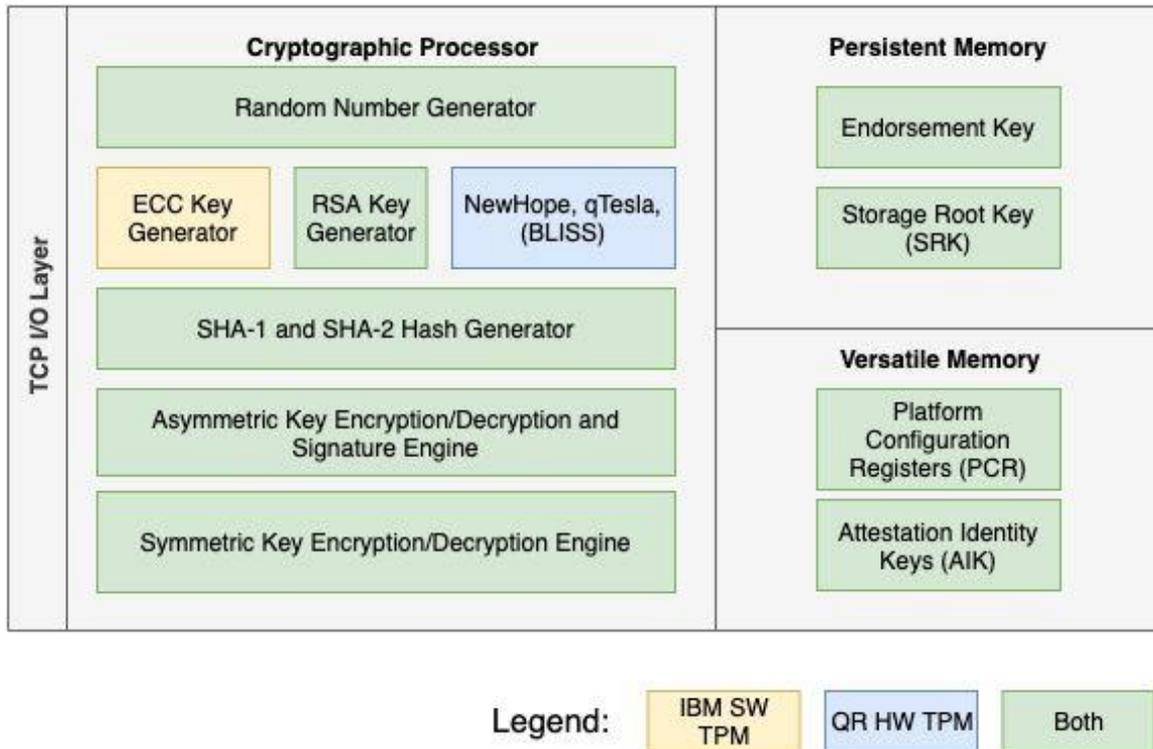
Figure 8: General overview of the QR HW-TPM and comparison to the IBM SW-TPM
