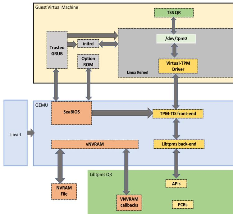
Figure 3: Architecture of V-TPM
