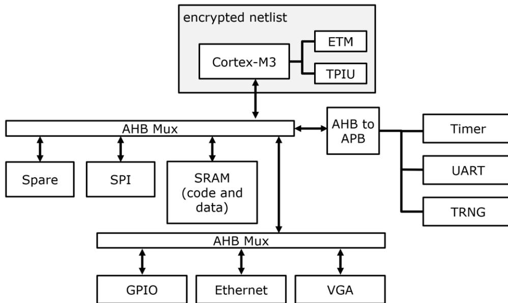
Figure 7: Simplified system overview on the DesignStart SoC
