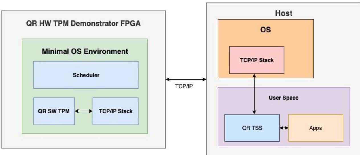
Figure 9: Block diagram of the QR HW-TPM demonstrator
