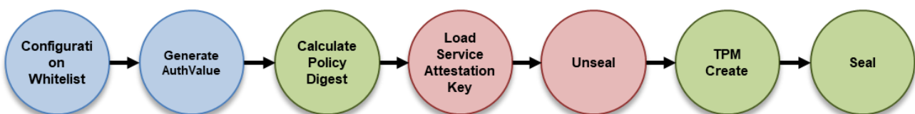
Figure 8: Diagram showing the states for generating an authentication key. Blue is provided by the host, green is states with relation to the authentication key and red is in regards to the service attestation (parent) key
